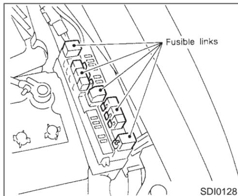
If any electrical equipment does not operate and fuses are in good condition, check the fusible links. If any of these fusible links are melted, replace only with genuine NISSAN parts.
