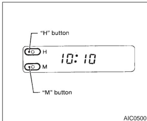
The digital clock displays time when the ignition key is in "ACC" or "ON".
