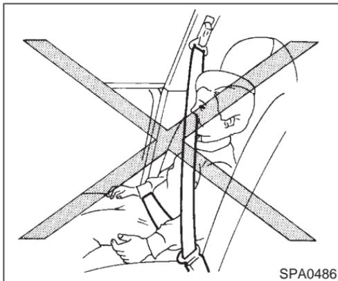
as possible **AROUND THE HIPS, NOT THE WAIST**. A lap belt worn too high could increase the risk of internal injuries in an accident.
