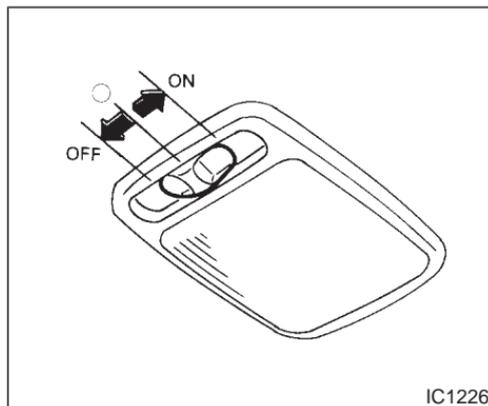
The interior light has a three-position switch.
