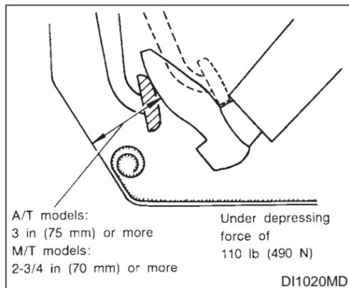
With the engine running, check the distance between the upper surface of the pedal and the metal floor. If it is out of the range shown above, see your NISSAN dealer.
