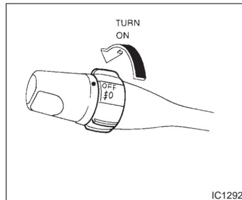
To turn the fog lights on, turn the headlight switch to the “ $\text{☉}$ ” position, then turn the switch to the “ $\text{☉}$ ” position. To turn them off, turn the switch to the “OFF” position.
