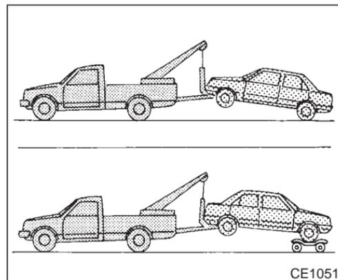
NISSAN recommends that your vehicle be towed with the driving (front) wheels off the ground as illustrated.
