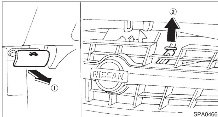
1. Pull the hood lock release handle (1) located below the instrument panel; the hood will then spring up slightly.
