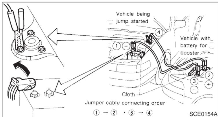
**Always follow the instructions below. Failure to do so could result in damage to the charging system and cause personal injury.**
