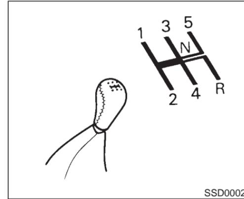
To change gears, fully depress the clutch pedal, then move the shift lever. After shifting, release the clutch slowly.
