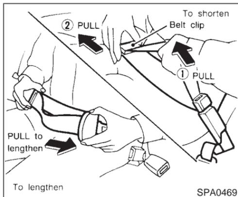
2. To lengthen, hold the tongue at a right angle to the belt and pull on the belt. To shorten, pull the end of the belt attached to the belt clip away from the tongue, and then pull the belt clip to take up the slack.
