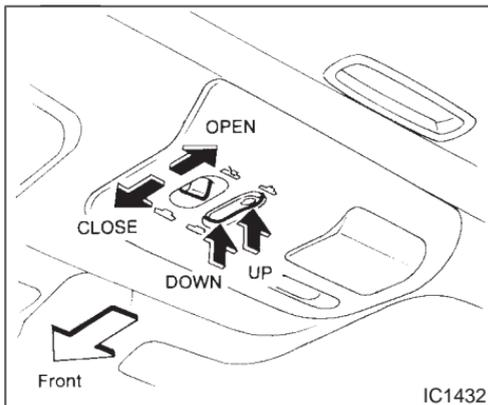
The sunroof will only operate when the ignition key is in the “ON” position.
