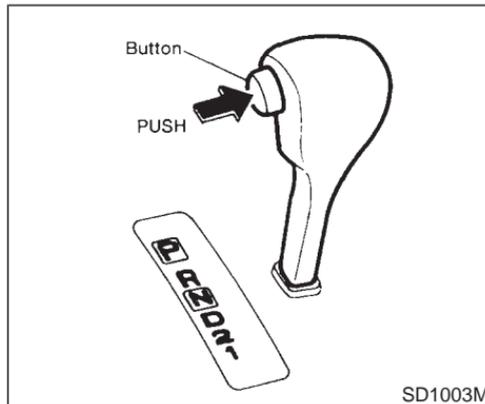
Push the button to shift into “P”, “R” or from “D” to “2”. All other positions can be selected without pushing the button.
