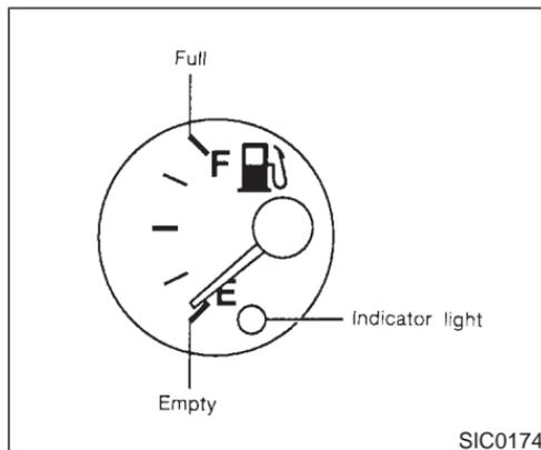
The indicator light comes on when the fuel tank is getting low. Refuel as soon as it is convenient, preferably before the gauge reaches “E”. There should be a small reserve of fuel in the tank when the fuel gauge needle reaches “E”.
