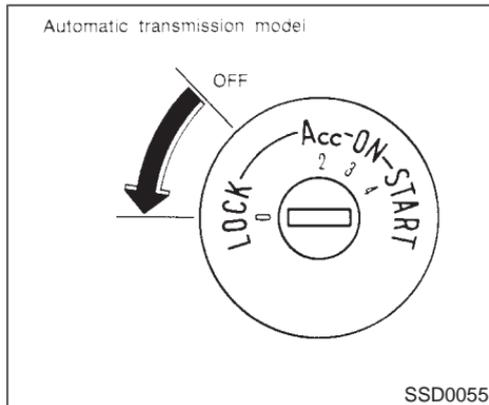
On automatic transmission models, the ignition lock is designed so that the key cannot be turned to "LOCK" and removed until the selector lever is moved to the "P" position.
