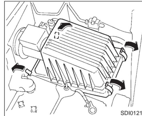
The filter element should not be cleaned and reused. Replace it according to the maintenance intervals shown in the "Maintenance schedule" section. When replacing the filter, wipe the inside of the air cleaner housing and the cover with a damp cloth.
