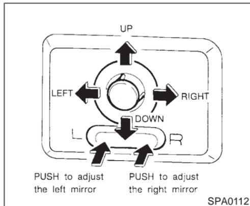
Push the right or left end of the switch to select the right or left outside mirror, then adjust using the control lever.
