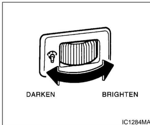
The instrument brightness control operates when the light switch is in the “ $\equiv$ ” or “ $\text{☉}$ ” position.
